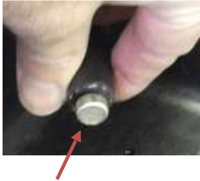
Intake Screen (On left hand side hose)
