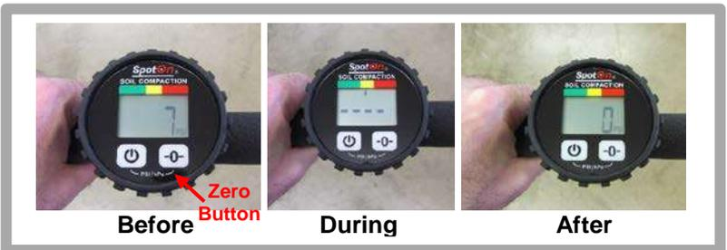
With the meter powered on, hold the meter above the ground with the shaft facing down. Press the **ZERO** button and continue holding the meter steady and above the ground until the zero function completes and the LCD displays a "0" value.
