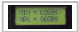
**SCREEN 3/4 & Up** - Pressing the START button additional times will allow the user to cycle through the readings held in temporary memory for each 1 cm of probing depth. These readings are only recorded for computer download if the logging function is ON. Once the max probing depth has been displayed the display will cycle back to the SCREEN 1 in a continuous loop. In this way you can always get back to a reading if you accidentally pressed the start button too many times.
