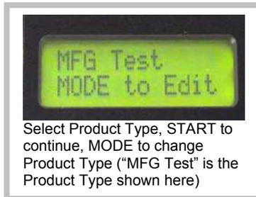
4.3.3 Once the START button is pressed again the meter will configure itself for a probing. Turning the meter OFF and then back ON will allow selection of a new Product Type and will reset all averages and standard deviation calculations.
