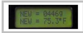
**SCREEN 2** - The multi-probe mean of both force and temperature for all probings since the meter was turned ON. The standard deviation is also displayed for all readings included in the mean (shown as the Greek symbol sigma). The meter will only calculate the mean and std dev for up to 6 probings. If more than 6 probings are taken without turning the meter off/on then the mean will show as 0. To reset this multi-probe averaging function turn the meter OFF then back ON.
