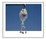
The meter comes with a reuseable "Nozzle Boot" to facilitate taking readings on irrigation nozzles. (See Fig. 1 and Fig. 2 above) Additional nozzle boots can be ordered from Innoquest by specifying Item # 26350.
