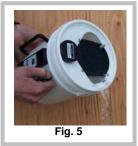
START button is pressed to start a new reading. Once the reading has been displayed, the water can be poured out of the meter (See Fig 5). Pouring out the contents of the meter will not affect the reading being displayed on the LCD. If a reading must be re-started for some reason, simply empty the meter and re-press the START button to ready it for a new measurement.
