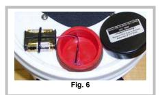
The batteries are housed under the black cap on the top of the meter. This black cap can be removed by pulling it straight up while twisting slightly. The cap is just a press fit onto the meter. The meter requires two (2) N size alkaline batteries which are
